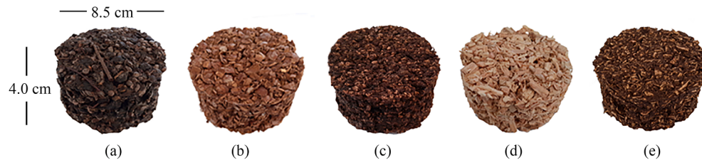
Fig. 4. Samples C – starch-based natural glue: (a) grape press waste (CG); (b) hazelnut shells (CH); (c) olive press waste (CO); (d) wood chips (CW); (e) wood chips and spent coffee grounds (CWc).
