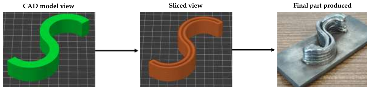
Figure 3.4. CAD representation vs Final part of geometry 3
