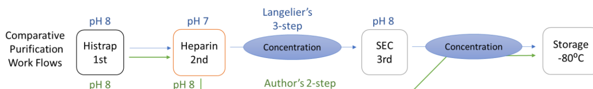
Figure 4.9 — Purification workflow. A schematic comparison of the 3-step (Langelier et al. [16]) and 2-step (Author's present work) PARP1 purification protocols.
