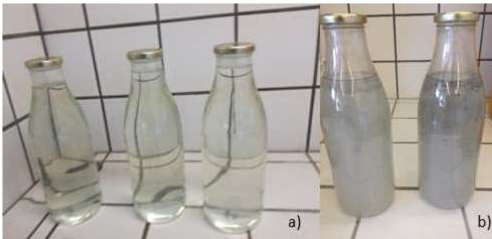
Figure 5.6 Photograph of stripped sour water samples in a) best-case scenario and b) worst-case scenario regarding suspended solids and oily matter content
