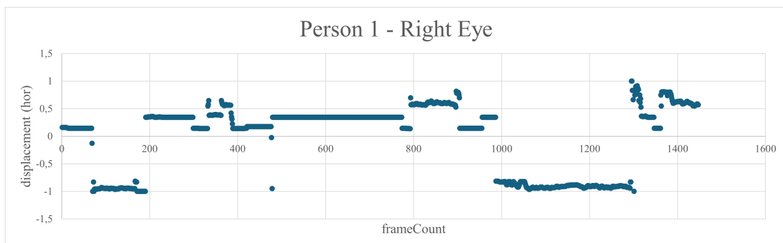
Figure 6.7: Graph of the horizontal position of person 1's right eye throughout the frames captured by the smartphone camera.
