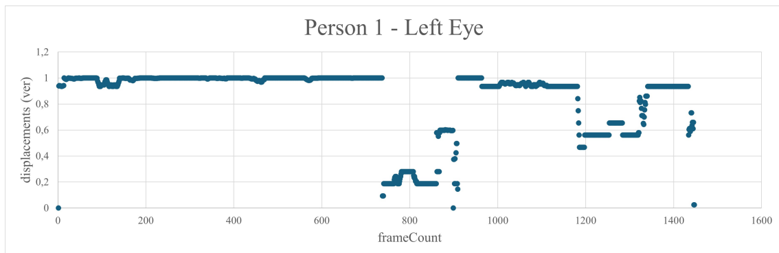
Figure 6.6: Graph of the vertical position of person 1's left eye throughout the frames captured by the smartphone camera.
