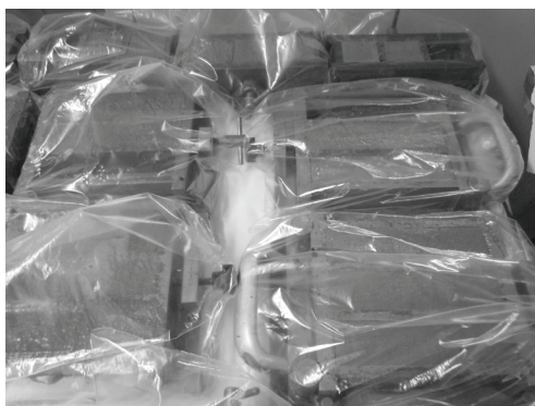
Figs. 4a and 4b Curing conditions for the specimens, source: M. Idália Gomes
