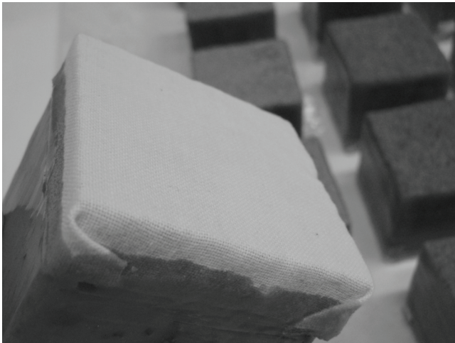
Figs. 6a to 6c Capillary water absorption, source: M. Idália Gomes
