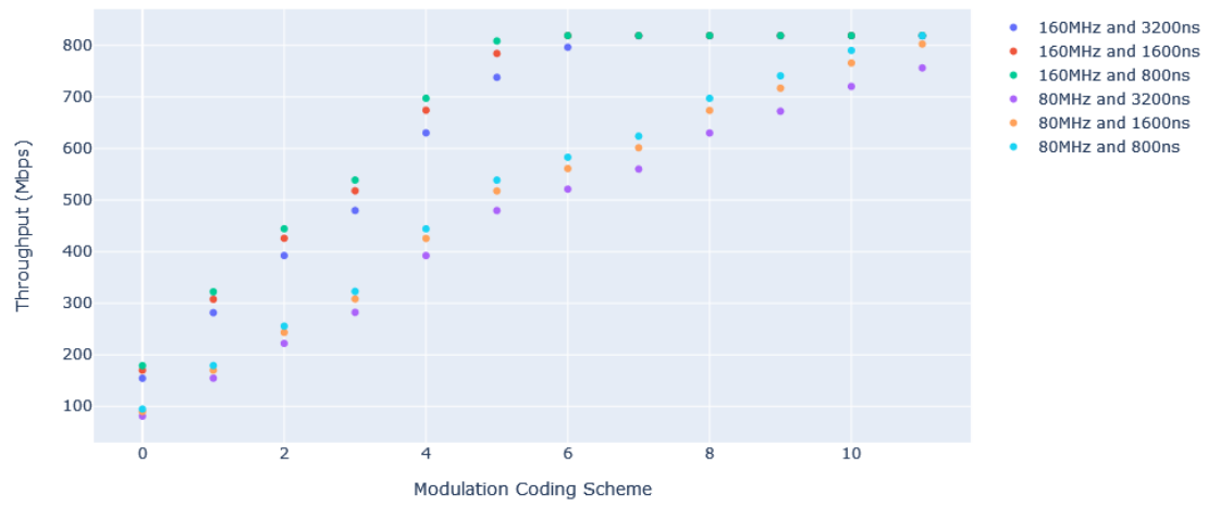
Figure 3.5: Throughput Across MCS for a GI of 800,1600,3200 ns and a Channel Width of 80,160 MHz
