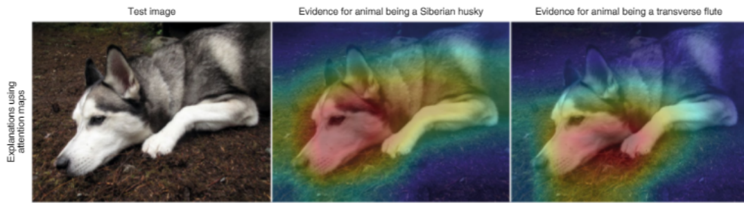
Figure 1.2: Saliency does not explain anything, it only shows us where the network is looking at. We have no idea why this image is labeled as either a dog or a musical instrument when considering only saliency. The explanations look almost the same for both classes. Credit: Chaofen Chen, Duke University [2].
