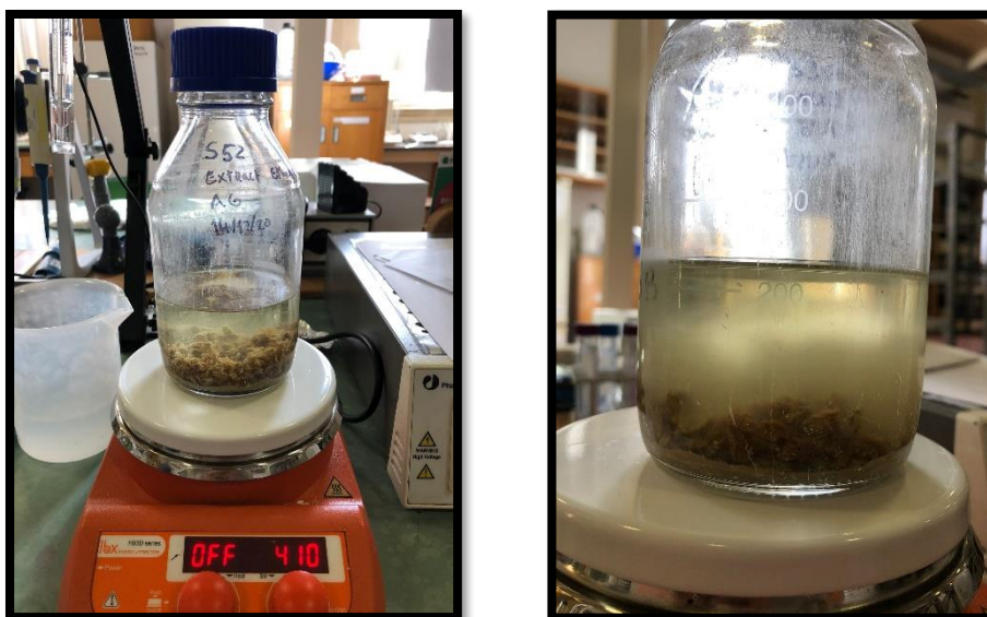
Figure 3.2 Maceration extraction method. The sponge inside a 500 mL shot containing 96% ethanol/ H 2 O (3:1). On the left, a stabilized viewing of the sponge inserted into the solvent and on the right, the same sponge allowing the perception of the extracts acquired. Afterwards, upon stirring, 25mL of the extract solution is retrieved to proceed with the experimental work.
