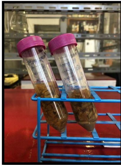
Figure 3.3 Total extraction method. Image of two falcons (50 mL), containing the sponge sample bathing in 96% ethanol for 30 min. Both falcons combined contained the total mass of sponge determined for this method, divided into two tubes, to achieve a greater sample- solvent contact area.
