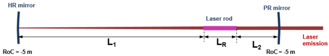
Figure 6.14 – Schematic diagram of the TEM 00 -mode beam propagation along the asymmetric laser resonator at side-pumping lasers with large RoC end mirrors. L_1 and L_2 represent the separation length of the high reflection (HR) mirror and partial reflection (PR) mirror, respectively, to the end face of the laser rod with length L_R .
