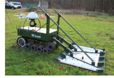
(c) UGV used for demining [16]
