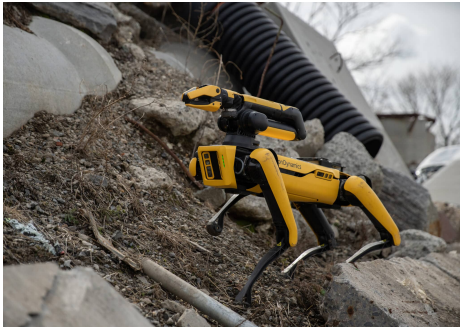
(a) Spot, a dog-like robot developed by Boston Dynamics 7
