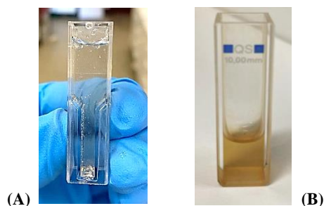
Figure 16 – Assays to assess the catalase-like activity of APTES SPIONs. (A) 5 \mu\text{L} of APTES SPIONs 5 \text{mg mL}^{-1} , 1 mL of phosphate buffer (10 mM, pH 7.4) and 20 \mu\text{L} of 0.88 M \text{H}_2\text{O}_2 . (B) Assay carried out using 10 \mu\text{L} of APTES SPIONs 5 \text{mg mL}^{-1} and 20 \mu\text{L} of 0.88 M \text{H}_2\text{O}_2 , in 1 mL of phosphate buffer (10 mM, pH 7.4), in a quartz cuvette.
