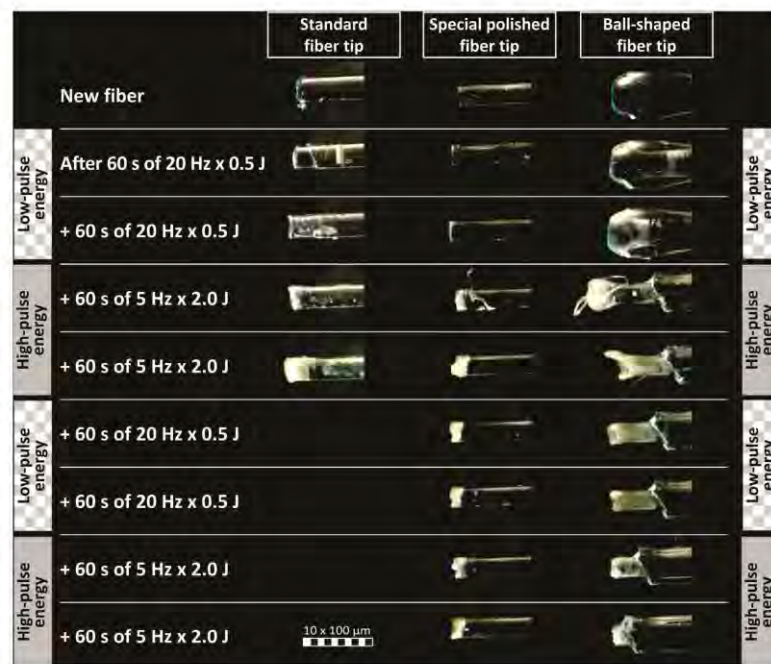
Figure 3. Microscopic analysis of fiber tip changed during course of experiments. Three tips showed minor tip changes after low pulse energy settings. When LoFr-HiPE laser emission was used, BT fiber showed intense degradation, which caused it to lose ball-shaped appearance, acquire menacing appearance and become undistinguishable from other fibers. PT fiber showed only cladding degradation and fiber tip opacification. Standard fiber was not subjected to gradual microscopic degradation analysis because it was always prepared again after each experimental run according to manufacturer instructions. Scale bar indicates 10 \times 100 \mu\text{m} .
