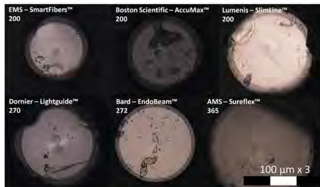
Figure 2. Light microscopy images of the tip of some of the fibers tested. This is the only way to visualize the innermost component of the fiber, namely, the core (seen as the bright inner disk). In some images, several layers of the cladding can be observed (seen as darker rings around the bright inner disk). The coating cannot be seen because it is out of focus. Note that the upper row of images relates to 3 fibers that are advertised as being 200 \mu\text{m} in diameter: the diameters of the cores are all different and the one to the right is clearly considerably larger than the diameters of the other 2 cores. Because most laser fiber information labels lack units or references to what the label numbers refer to, units were also omitted for each fiber of this figure. (Color version available online.)
