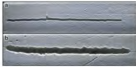
Fig. 2 Comparison of the results of different lithotripter settings using the same total power level (6 W) and the same laser fiber (200 \mu m fiber core). a Uses a high-frequency and low-pulse energy (HiFr-LoPE) at 30 Hz \times 0.2 J, while b employs a low frequency using high-pulse energy (LoFr-HiPE) at 5 Hz \times 1.2 J
