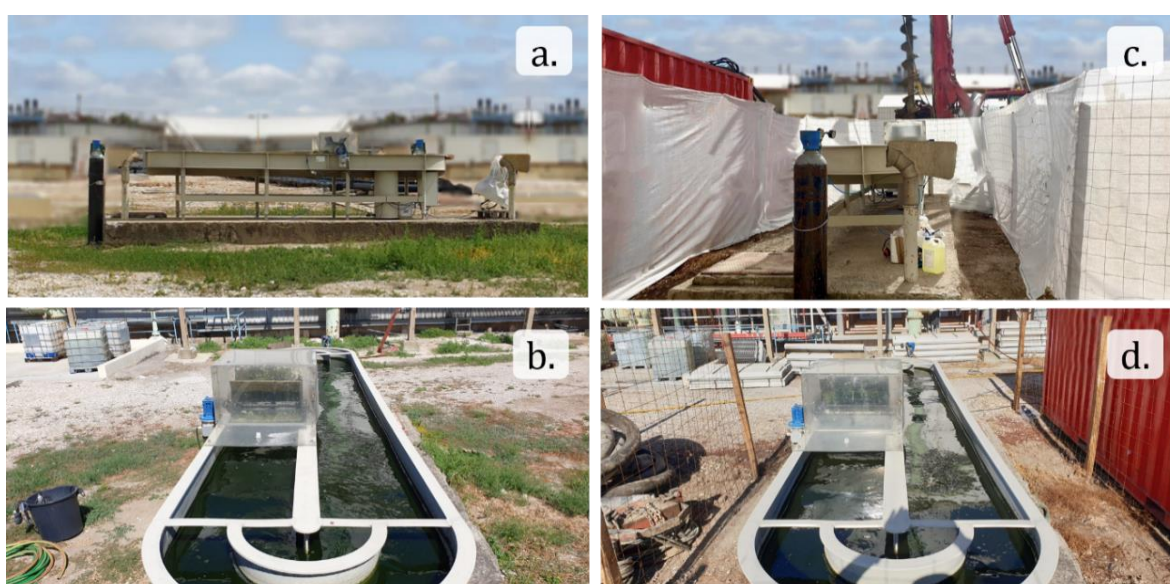
Figure 5.3 – Raceway used for this assay. Photographs a. and b. represent the typical disposition of the bioreactor in the industrial site. Photographs c. and d. were taken in September 2021, when construction work was initiated and is still ongoing.
