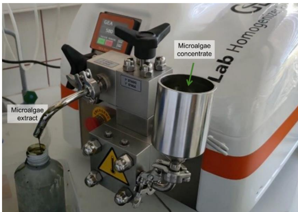
Figure 4.5 – High-pressure homogenization process (GEA Lab Homogenizer PandaPLUS 2000).
