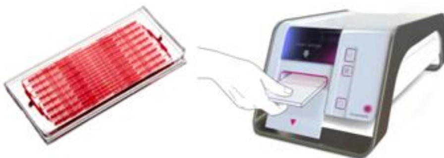
Figure 5 | Illustration of circulating tumour cells isolation cartridge and equipment (adapted from RUBYnanomed Business Plan).
