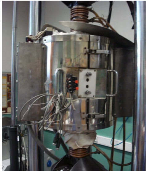
Figure 2.4: Servo-hydraulic machine and furnace used to perform the axial tensile and fatigue tests
