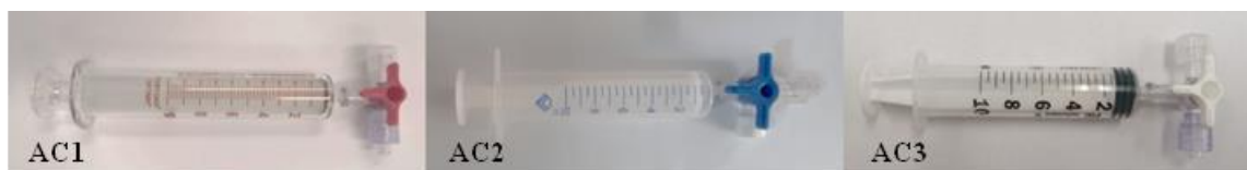
Figure 23 - Syringe-based air containers (AC) used in this study, namely, full glass (AC1, left), plastic with plastic plunger (AC2, middle), and plastic with rubbered plunger (AC3, right) [10].
