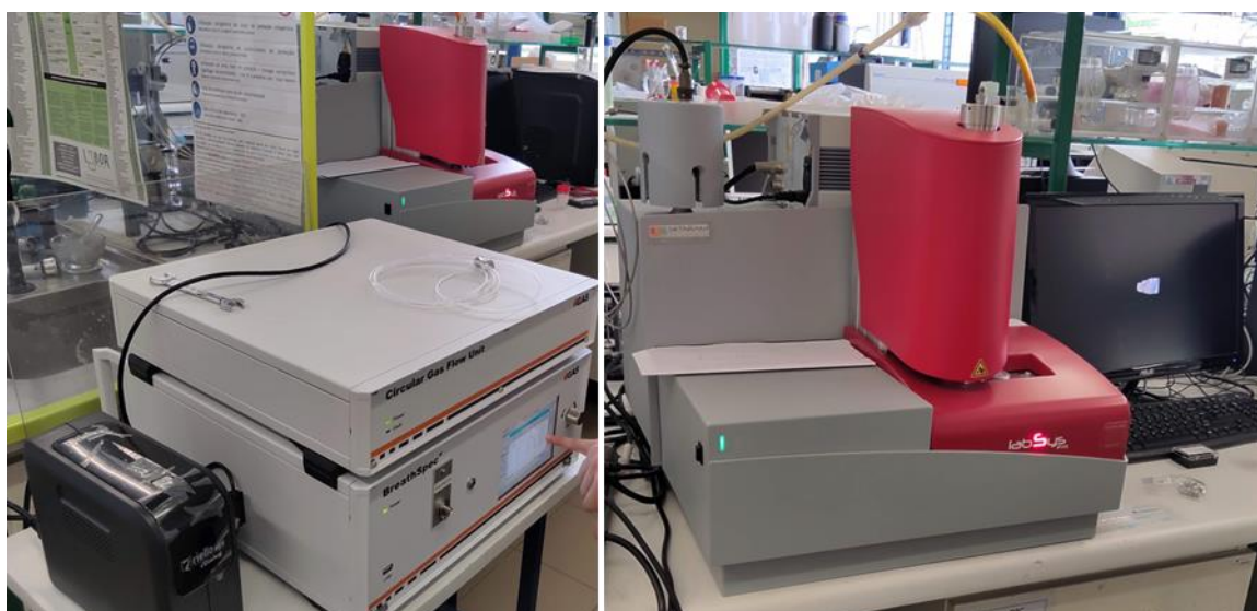
Figure 19 - GC-IMS coupled with a GCFU unit working in parallel with the TGA device (left), and the TGA device by itself (right).
