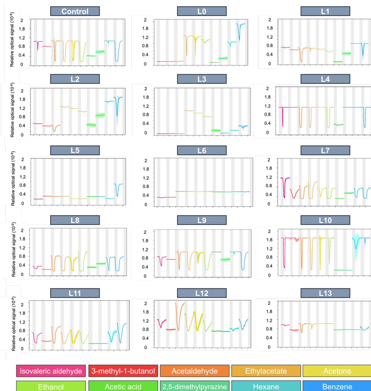
Figure S5.5 – Representative signals of the optical amplitude responses in optical e-nose experiment, of control and all ligands-hybrid gels sensors, to the set of 10 distinct mVOCs tested. Each curve represents the average and standard deviation of at least 19 replicate cycles from the same sensor. VOC exposure periods (5 s) are highlighted in grey, and each cycle corresponds in total to 15 s. The plots were generated by python.
