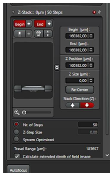
Figure 2.1: Z-stack dialogue box with the begin, end and number of steps options shown. (Selected options shown in red).
