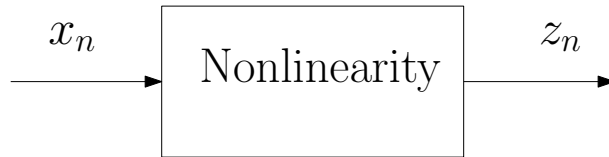
Figure 2.2.3: Block diagram of bandpass memoryless non-linearity.
