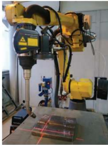
Figure 2.14: Integration of the FANUC iRVision 3DL system into a welding robot for surface defect detection [31].
