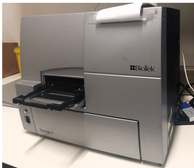
Figure 2.3: Synergy™ 2 Multi-Mode Microplate Reader (BioTek) used for experimental assays, with the microplate carrier open.
