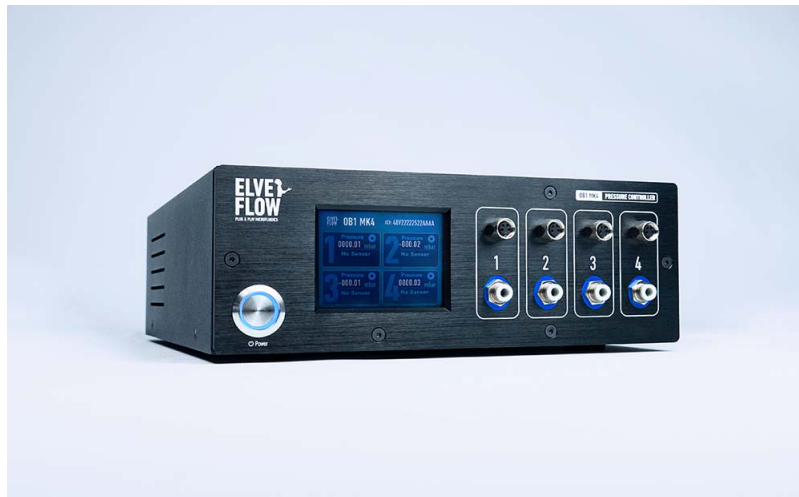
Figure I.1: Elveflow® OB1 MK4 pressure and vacuum controller. As input, an external pressure (air compressor, local pressure network or gas cylinder) or vacuum source needs to be connected. It features a USB entry allowing pressure monitoring and sequence automation using a dedicated software. It pressurizes up to four reservoirs and can also connect to up to four flow sensors at the same time. It uses piezoelectric technology which gives more precise and faster flow control than other technologies available in the market. Mainly, its advantages are that it has a fast settling time (around 40 ms) and a highly stable and pulseless flow. Adapted from [97].
