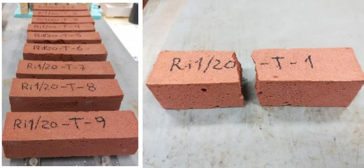
Figure 3.1. Clay-based mortar samples: (a) when drying; (b) after flexural test.
