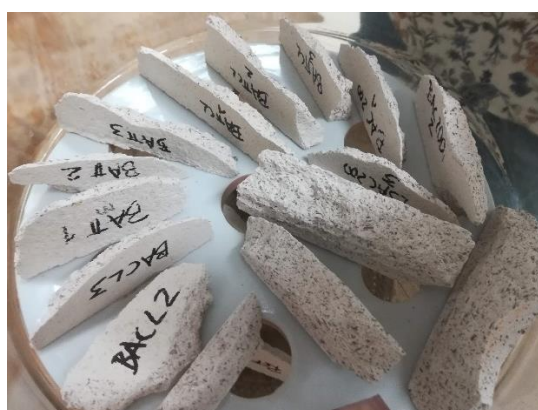
Figure 5.2. Samples collected from plasters applied on bricks (a) and from prismatic specimens (b) that underwent vacuum and hydrostatic weighing open porosity test.
