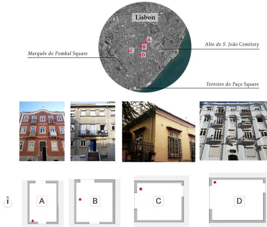
Figure 2.2. Selected case studies: location in the map of Lisbon, building facades, and plans of the monitored bedrooms (openings: interior door and outdoor-facing window). In each room, a red dot indicates the position of the data-logger used to monitor the indoor hygrothermal conditions.
