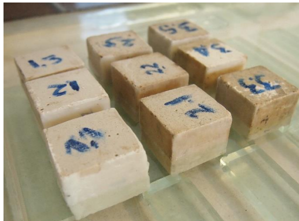
Figure 4.12. Specimens during water absorption by capillarity test: 1 – reference mortar; 2 – flowers at 5%; 3 – leaves at 5%.
