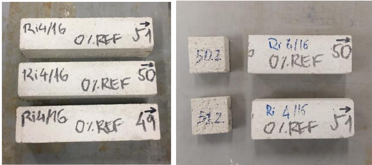
Figure 3.2. (a) Prismatic samples of C 1.3 ; (b) sliced to obtain specimens 40x40x20 mm 3 .
