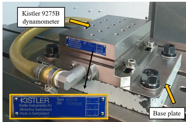
Figure 4.6 Kistler 9257B dynamometer
