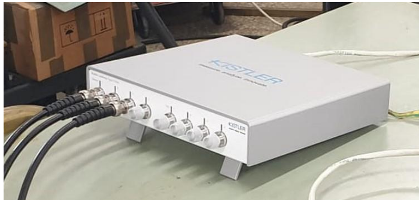
Figure 4.7 Kistler LabAmp 5165A charge amplifier & DAQ
