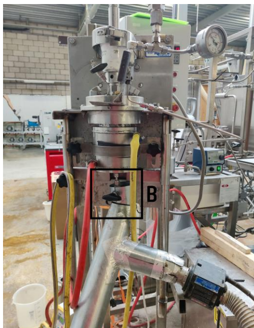
Figure 3.4 PGSS apparatus (Valve B (NV-03) – sprayed microparticles)
