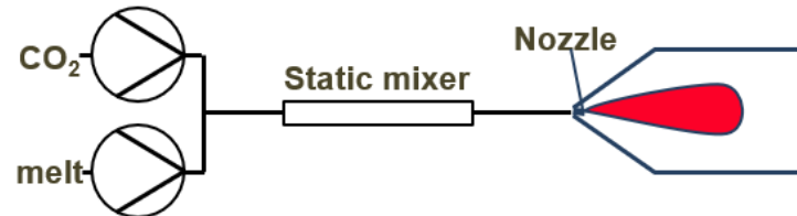
Figure 2.5 Scheme of the PGSS process in batch and continuous mode (with permission of Feyecon Development in the Netherlands)
