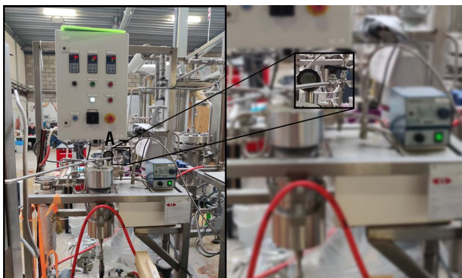
Figure 3.3. PGSS apparatus (Valve A (BV-03) – Injected CO 2 in the system)
