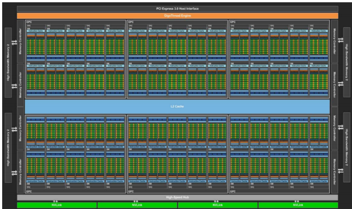
Figura 2.1: GPU Pascal GP100 completa, com 60 SMs
