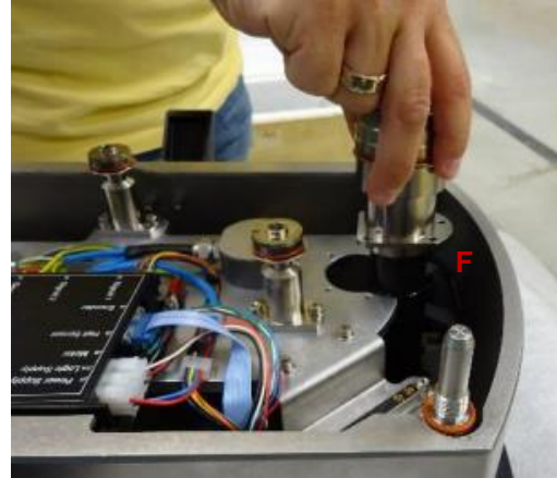
Figure 1.8 – Gearbox being assembled on the weighing scale box; F – Gearbox [33].
