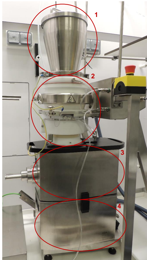
Figure 1.5 – GEA Compact Feeder fully assembled. 1 – External hopper; 2 – Topup system; 3 – Greenhouse; 4 – Weighing scale box.
