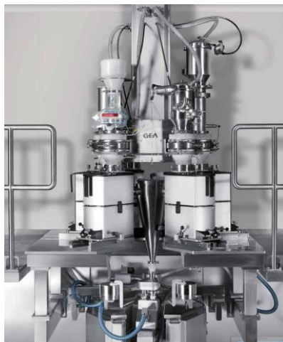
Figure 1.2 – Demonstration of a join of GEA Compact Feeders feeding into the continuous line [15].
