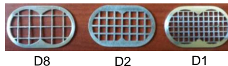
Figure 1.13 – The three meshes available to set on the feeder [26].
