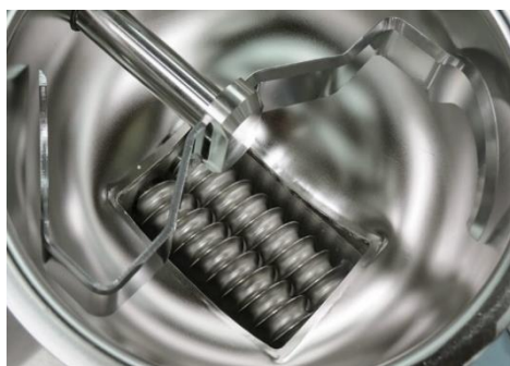
Figure 1.4 – Horizontal agitator on KT20 Feeder’s bowl [34].
