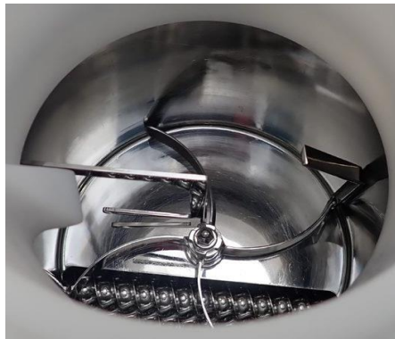
Figure 1.3 – GEA Compact Feeder's hopper with an asymmetric agitator and baffle set.
