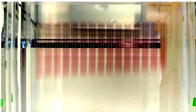
Figure 3.17: Result of the sum of all the analysed frames of a video. Contrast was enhanced to provide better visualization of the lanes. The background is clearer and without obstructions, possibly improving the results.
