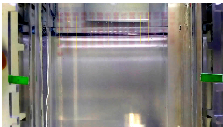
Figure 3.23: Result of the sum of all the analysed frames of a video. Contrast was enhanced to provide better visualization of the lanes. The starter point of the lanes was identified and all the lines with different start were discarded. Each yellow line represents the lane that was created by aligning the centers of the bands/wells.
