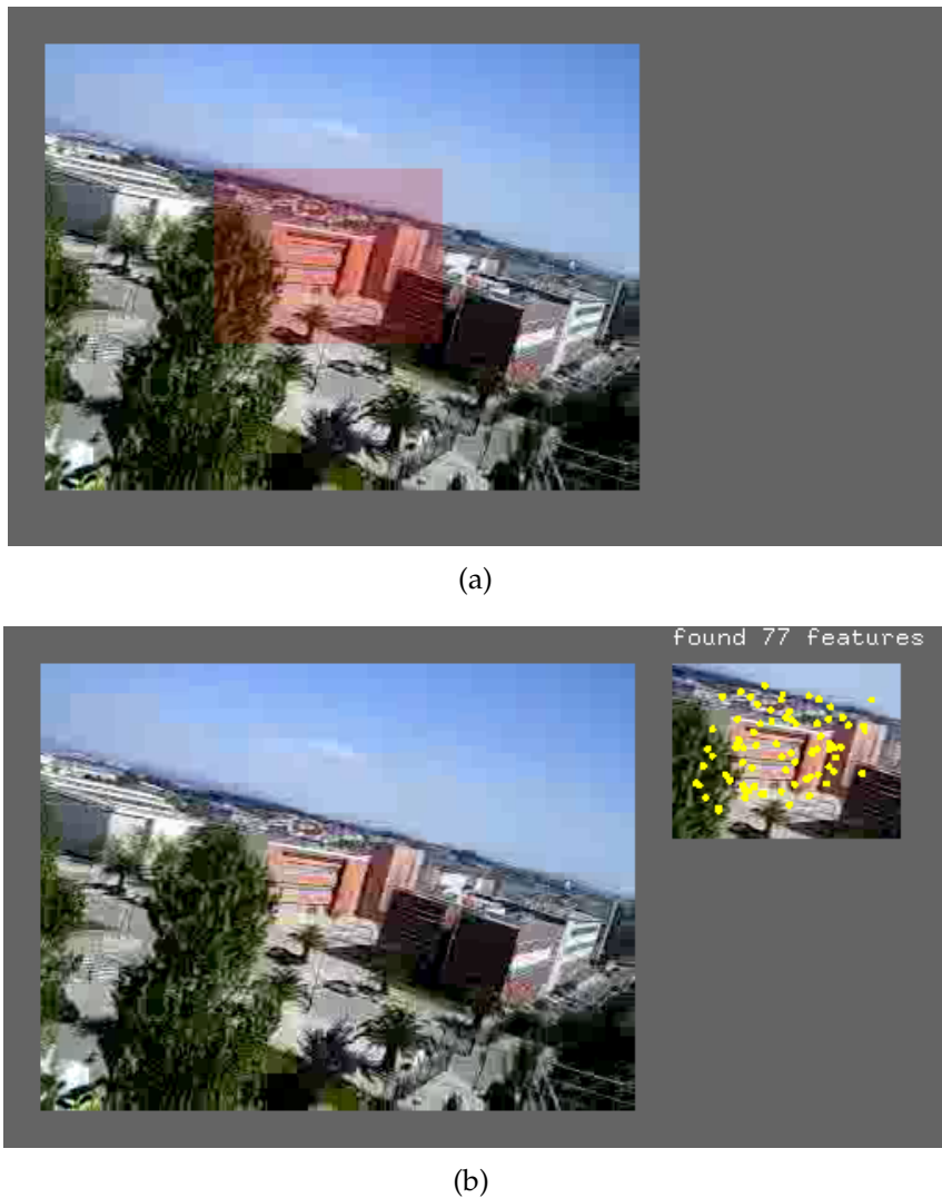
Figure 3.13: Prototype snapshots [NC12c]. Panoramic video of a campus taken from the roof of a building. The camera was tilted and rolled to make detection more difficult. In (a) a building is selected. In (b) the SURF descriptors of the selection are extracted.
