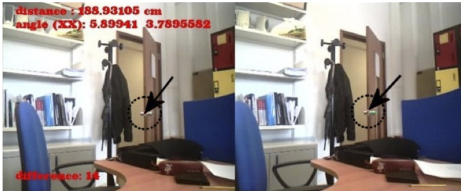
Figure 3.15: Interactive prototype to roughly measure the distance of a point chosen by the user to the camera on the left image. The camera parameters must be known for this stereo view method.
