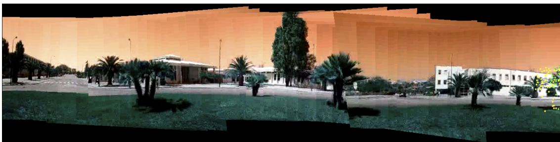
Figure 3.12: Prototype for fast creation ( \sim 5 fps) of panoramic scene from a continuous video sequence using flow detection to calculate the homography and the respective rotation of the images.
