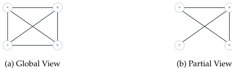
Figure 2.1: Comparison between global view and partial view on a P2P system network
