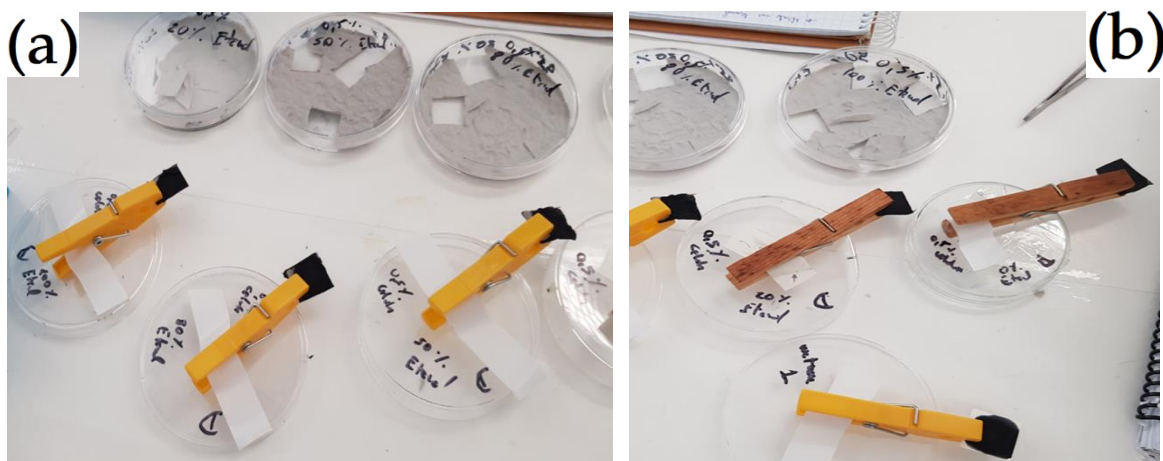
Figure A.8 — (a) (b) Photos of recycled paper substrates with: 20% Ethanol; 50% Ethanol%; 80% Ethanol that are being left to dry and their respective boxes contacting the paper used.
