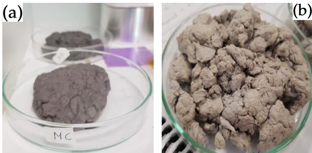
Figure A.4 — (a) End product after filtration and before putting it in the oven again (b) Dried cellulose
