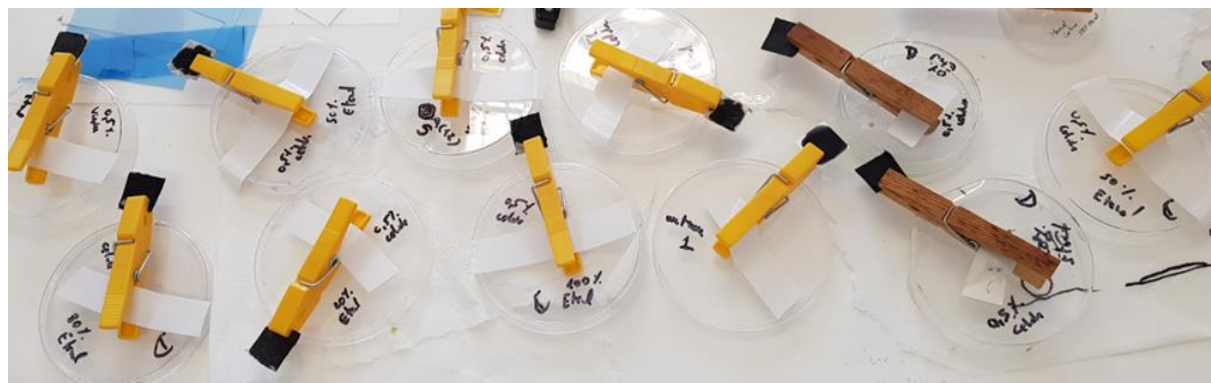
Figure A.7 — Multiple recycled paper substrates with varying degrees of Ethanol being left to dry after functionalization with PPy.
