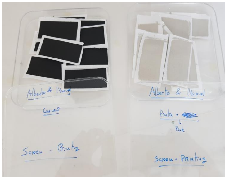
Figure A.13 — Picture of the final paper obtained through the Screen Printing process. The left ones are of Coal and the right one is of Silver
