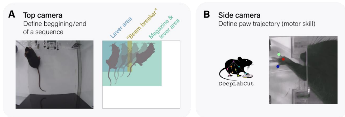
Figure 8 – Top and side camera data analysis. (A) Different areas of the box were defined on Bonsai, as well as the centroid of the mouse, allowing mouse tracking to define lever press sequences; the end of a sequence was defined as the last lever press prior to crossing the “beam breaker”, while the beginning of a sequence was defined as the first press after the end of the prior sequence. (B) Side camera data was used to estimate paw trajectory using DeepLabCut. Forepaw labelling: paw centroid in red, first digit in blue and fourth digit in green.
