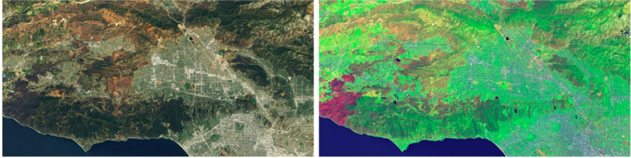
Figure 3: Example of satellite imagery for forest fire scar identification. Standard true-colour image (left) vs shortwave infrared (right), revealing extent of fire damage (NASA 2021)
