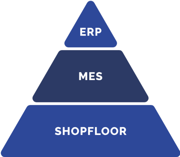
Figure 6 - Hierarchy of Manufacturing Systems based on (D' et al., 2017)
