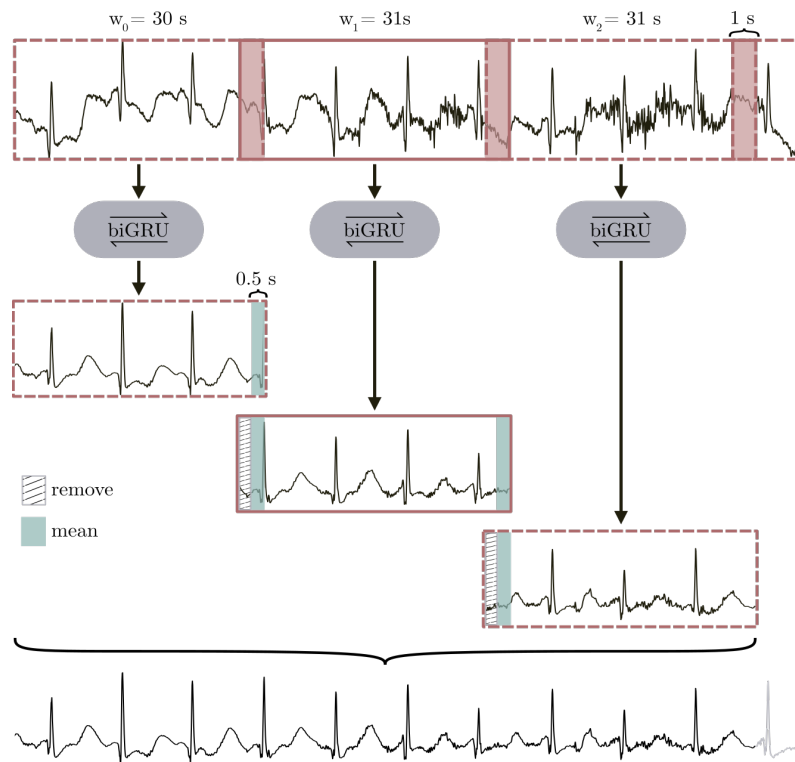
Figure 5.3: Illustration of the segmentation process applied to long ECG signals. Within the reconstruction phase of the process, "remove" and "mean" correspond to two key actions performed on output signal segments: "remove" indicates the portions of the signal that are cut, while "mean" designates the segments overlapped to compute the final reconstructed signal, depicted at the bottom of the figure.
