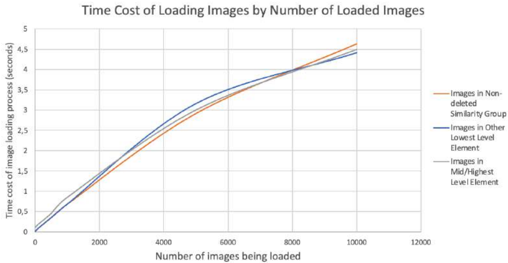
Figure 4.6: Plot representing the results obtained by the practical tests performed to validate the time complexity of the function used to load images.
