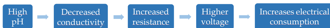
Figure 4.4. Expected relations between pH and conductivity with electrical resistance at the catholyte.
