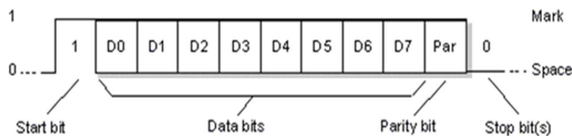
Figure 3.16 - Transference of data in the UART protocol. [113]
