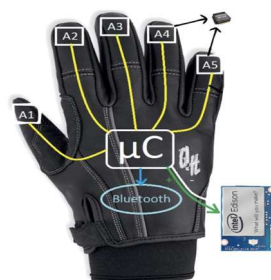
Figure 3.6 - Sensing glove based on IMU sensors developed in [82].
