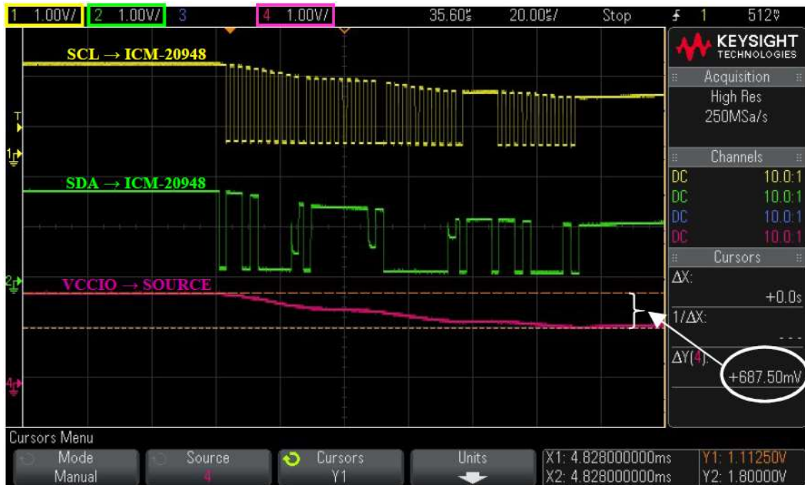
Figure 5.4 - I 2 C communication signals: SCL (ICM-20948) in yellow; SDA (ICM-20948) in green; VCCIO (source) in pink.
