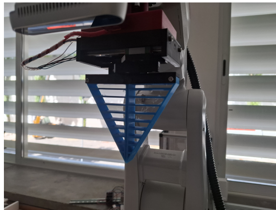
Figure 4.3: Image of the complete assembly of the first version of fin ray gripper assembly
