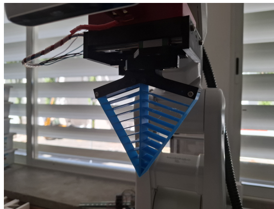
Figure 4.8: Image of the complete assembly of the second version of fin ray gripper assembly
