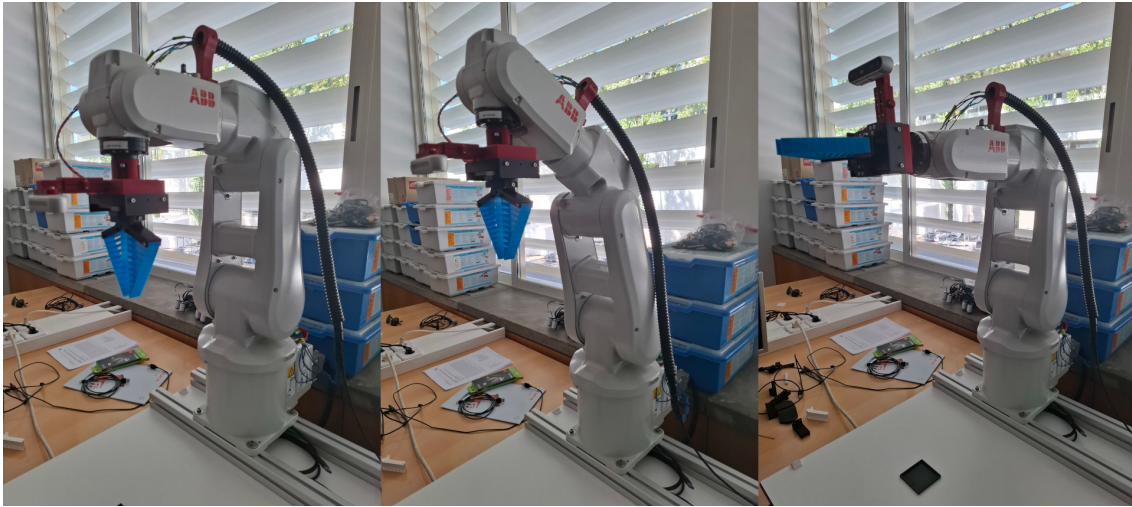
Figure 6.3: Three robot's hard coded positions (from left to right: home position, upper home position, calibration position)
