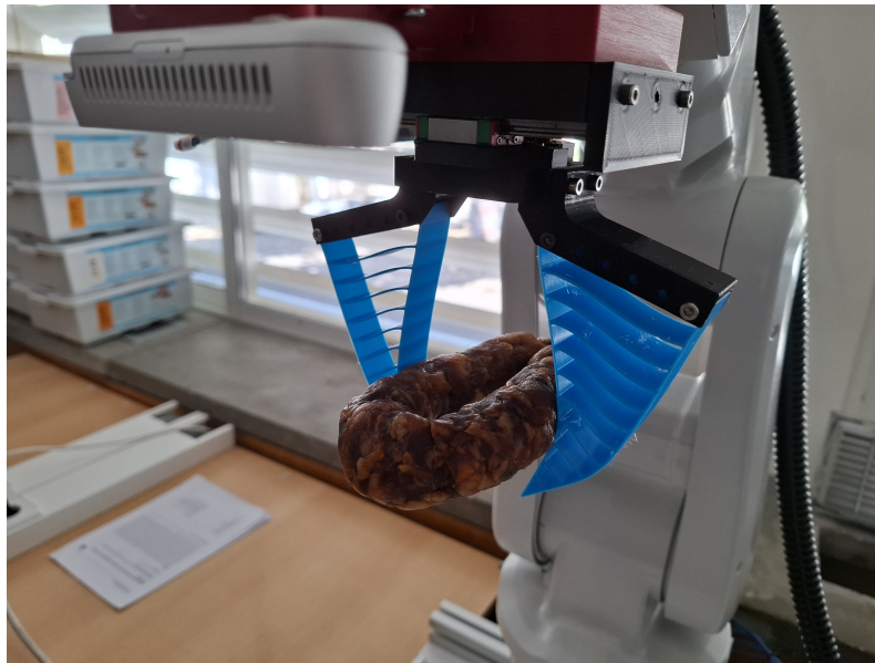
Figure 7.1: Successful fin ray effect gripper agri-food grasp
