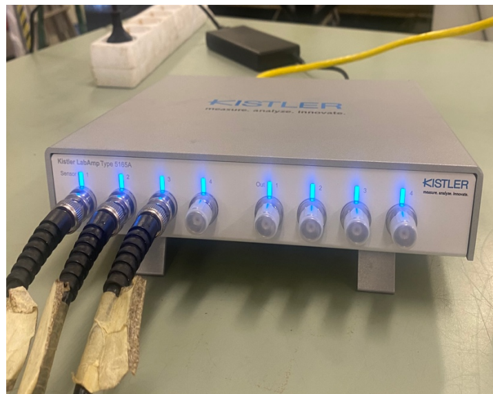
Figure 3.10 - Kistler LabAmp Type 5165A charge amplifier with integrated data acquisition.
