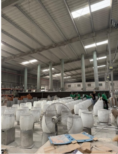
Figure 57: Workers creating stools out of cement by hand (own picture)
