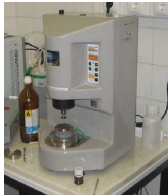
Figure 3.22: Main parts in the rotational rheometer used in the present work: (a) gap size indicator; (b) device to determine the shear rate (or stress) response and a device to apply a constant torque (or rotation speed) to the tool, respectively; (c) measurement tool; (d) thermostatic bath with temperature control.
