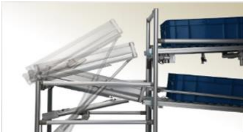
Appendix 8 - ModulPipeSmart -system, the "Flip Flop solution"
