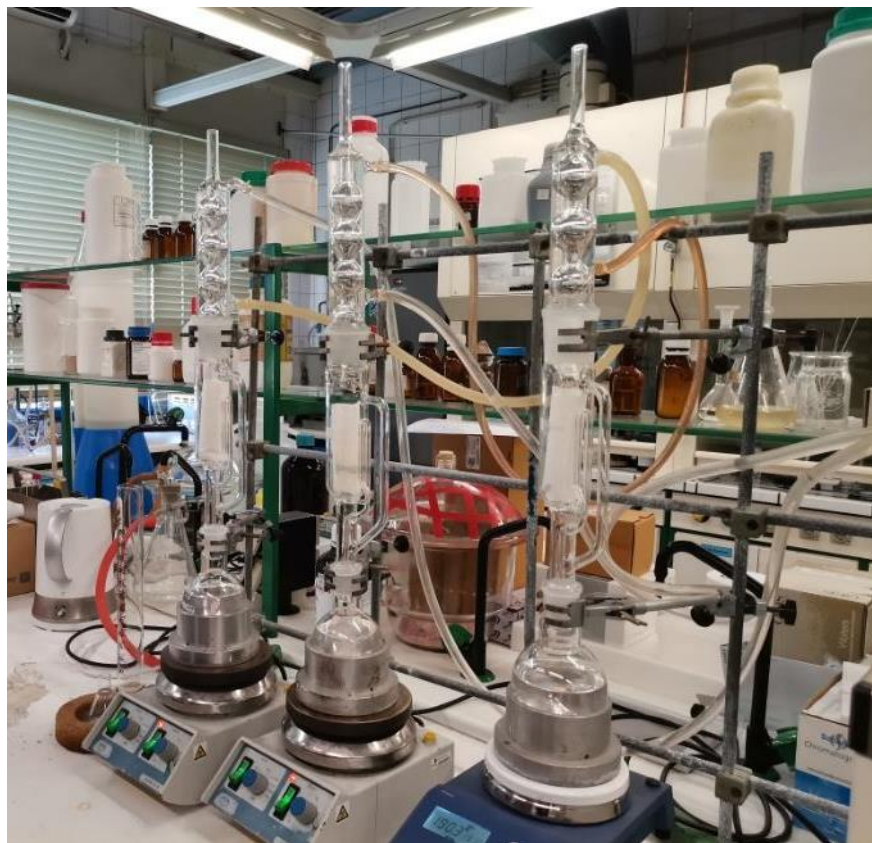
Figure 12 - Soxhlet apparatus for the extraction of selected seaweeds.
