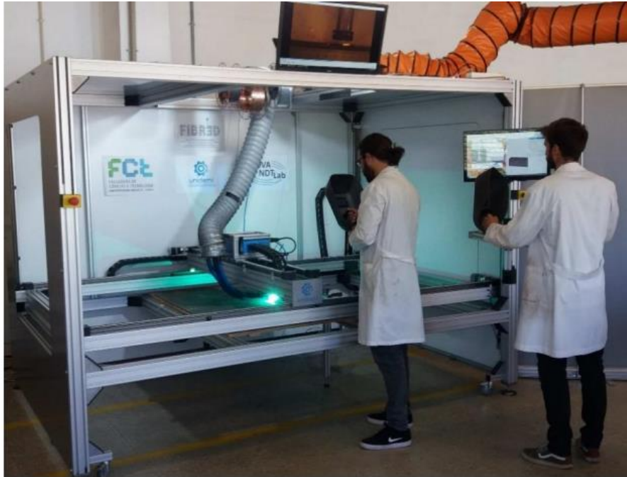
Figure 3.2 - Motion system 3 axis [17].
