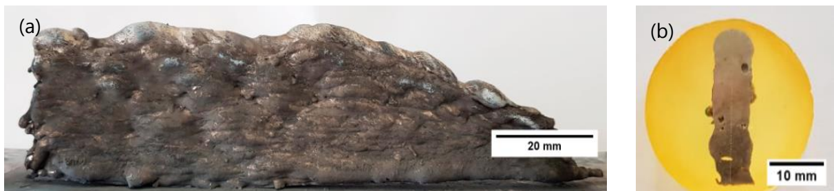
Figure 3.5 - Schematic representation of the preparation of samples for microscopy; (a) slice used; (b) sample in resin.
