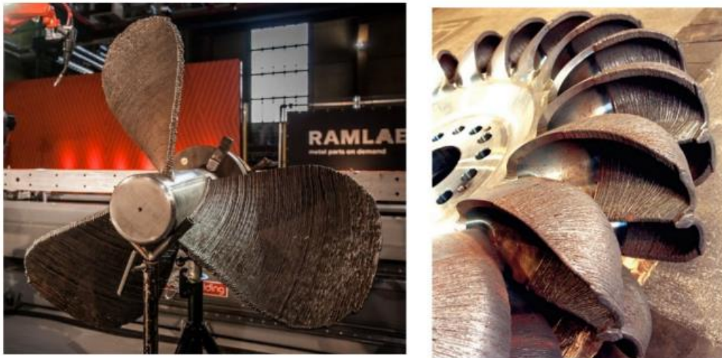
Figure 2.7 - (Left) WAAM-manufactured propeller; (Right) WAAM-manufactured Pelton turbine blades [7].
