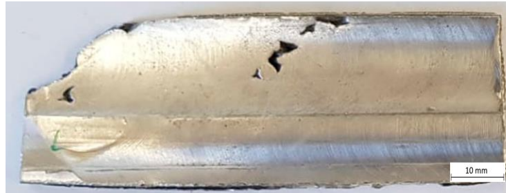
Figure 3.7 - Machined deposited wall.
