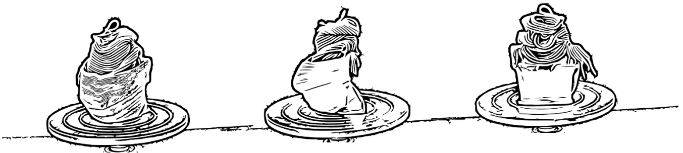
Figure 3.4.9 - Drawings of a printed model in BT clay without support
