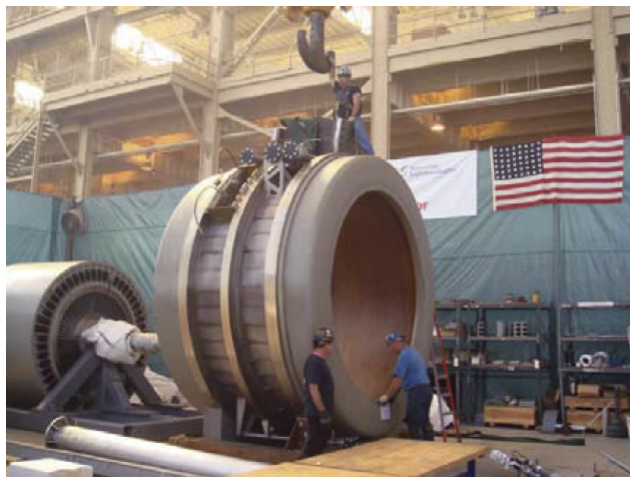
Figure 2.29: 36.5 MW synchronous motor manufactured by AMSC (Gieras, 2009).
