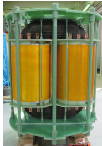
(b) Nakoya University YBCO single-phase transformer (Kotari, Kojima, Hayakawa, Endo, & Okubo, 2010).
