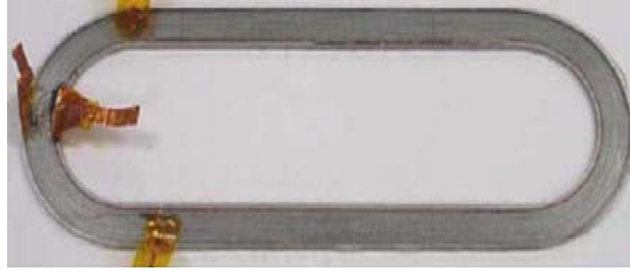
Figure 2.38: HTS rotor excitation winding (Gieras, 2009)
