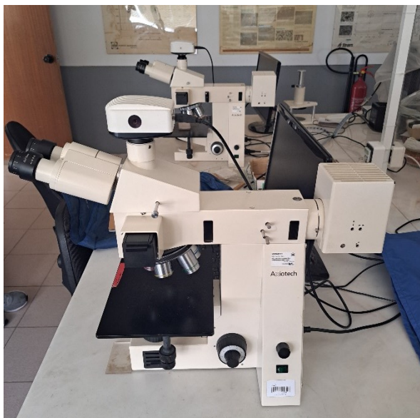
Figure A.5 Axiotech microscope with a Zeiss infinity 2 digital camera.
