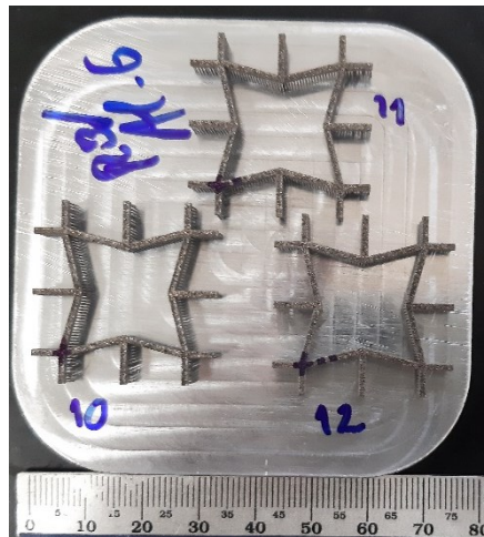
Figure D.10 Practical example of the samples 10, 11 and 12 for the parameters' optimization of AlSi10Mg.
