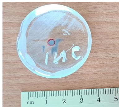
Figure 3.5 Inconel 625 powder embedded in polished Epoxy resin.
