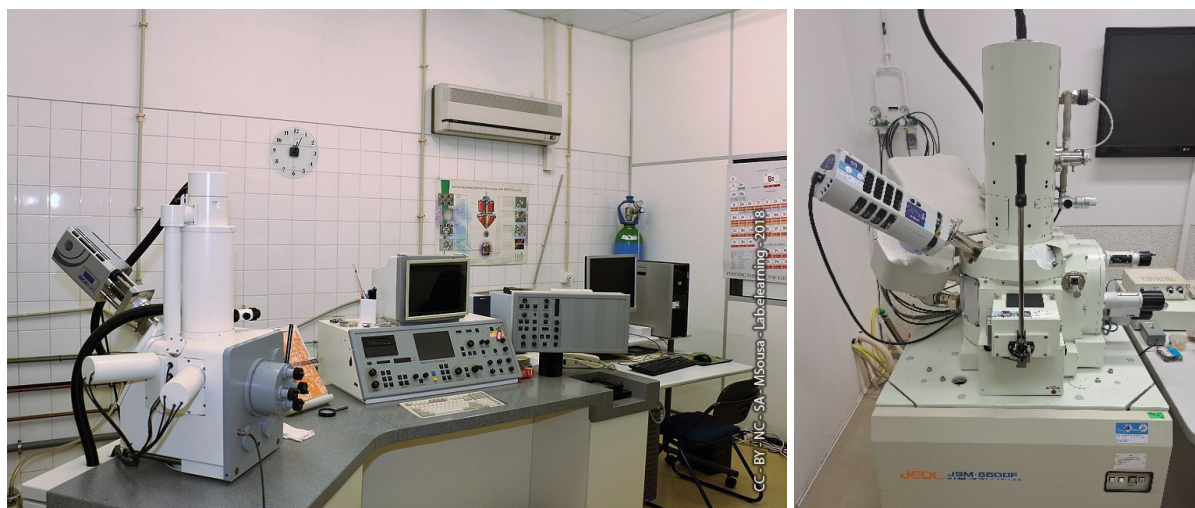
Figure A.6 Scanning electron microscopies used. A) Zeiss DSM 962 at NOVA (Source: CENIMAT website ); B) JEOL, JSM-B500F at ISQ facilities.
