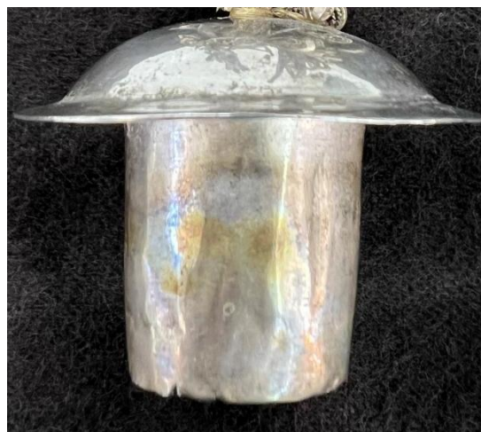
Fig. 6.12 Silver alloy corrosion having different color variations aligning with the corrosion pattern of sterling silver
