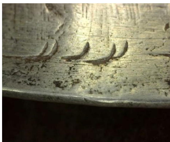
Fig. 6.5 Chasing marks, showing several identical tool marks in terms of shape and dimension probably attributed to the use of a specific punch tool
