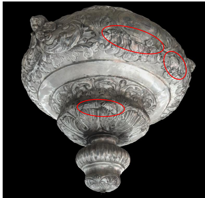
Fig. 6.17 3D scanning pictures of the ecclesiastical lamp revealing the areas which have several patches performed during the use of the object that cover cracks
