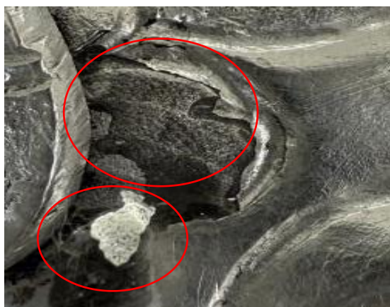
Fig. 6.23 Metal detachments, observed during the inspection of the piece
