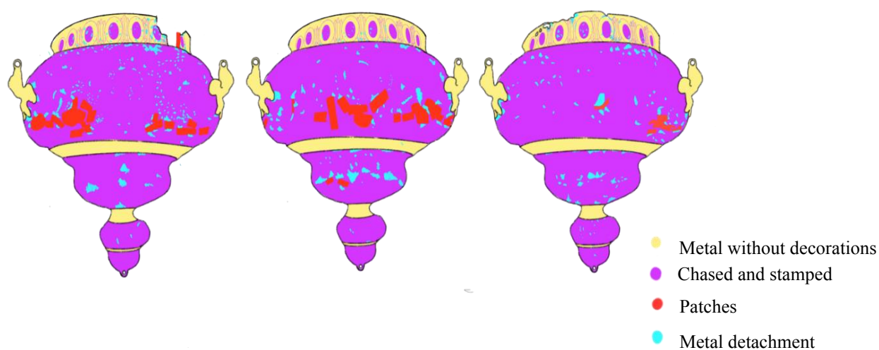
Fig. 6.24 Mappings with the patched areas and metal detachments of the lamp, highlighting the position of the detachments compared to the patched areas
