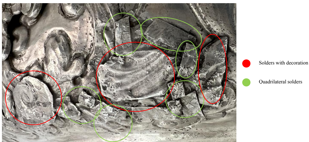
Fig. 6.20 Repair patches performed on the lamp, having distinct shapes, the red ones being made using repoussé and chased decoration technique, and the ones highlighted with green have no decorations, showcasing the difference between patches
