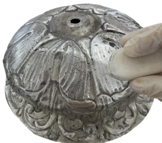
Fig. 6.25 Image with the lamp cleaned using the eraser, showing the efficiency in tarnish removal in the brighter area
