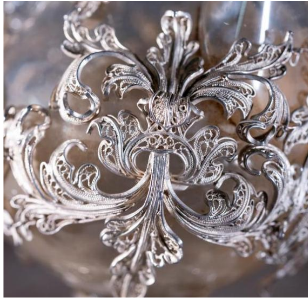
Fig. 6.10 Vegetal decoration silver alloy filigree of the cruets, offering insights on the manufacturing solders and shapes
