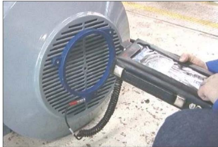
Figure 3.12 - Equipment used to measure the axial flux in an electrical machine [97]
