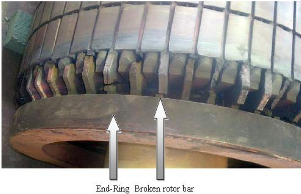
Figure 2.8 – Fabricated rotor of a 5 MW rated power ( P_{el} ) machine with multiple broken rotor bars [65]
